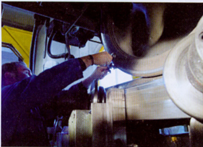
Fig. 1. Degree of wheel wear measured along the reconditioning pit
